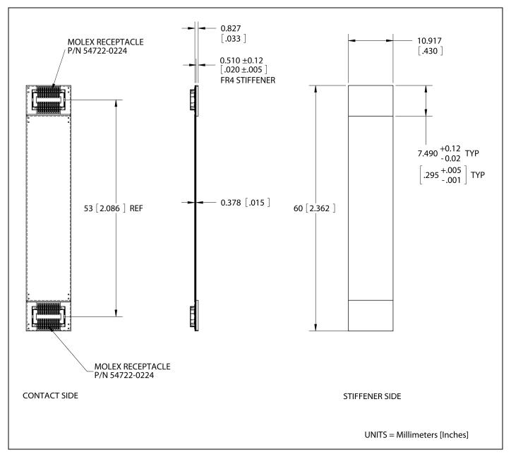
Figure 38. Flex Cable Dimensions, P/N 77-77104
